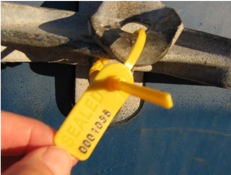
Plastic Seal tail shall be at least 1 inch long - pull tail through until it clicks at least once
