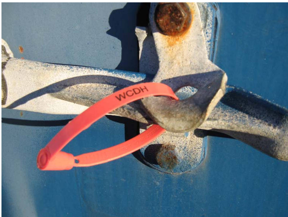
Plastic Seal end shall be clicked into the socket at least once
